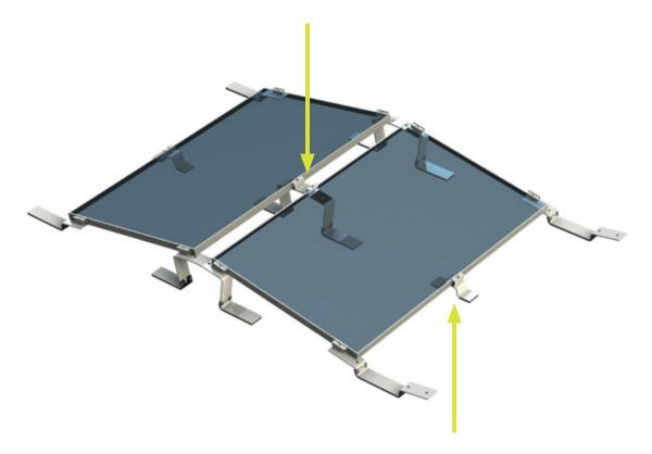
Position a Bottom part in the centre of the module using an end clamp and screw it tight.
