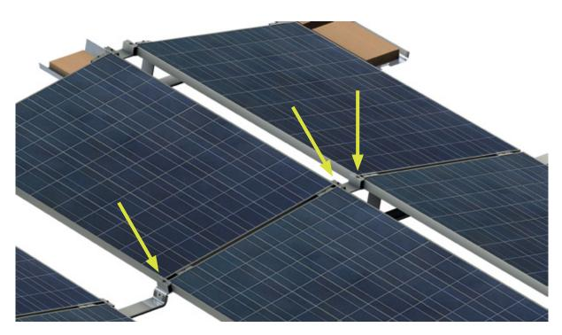
Attach the additional end clamp at the top of each Top Parts and Bottom Parts. An additional clamp is not necessary for the Front Part at the start and end of each row.
