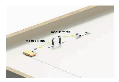
Place the Front Parts, Top Parts and Bottom Parts at approximately the required horizontal distance (module length). The exact distance is adjusted during installation of the modules.
